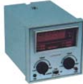
LS96-2211(IN-030) Feature Double potentiometers upper and lower limit setting, number indicating thermoregulator Outlook Dimension 96X96X130mm Hole Dimension 92X92mm
